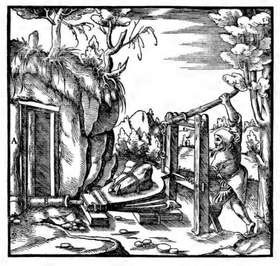
A-TUNNEL. B-PIPE. C-Nozzle of double bellows.
